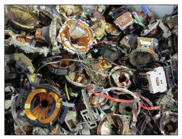
Picture 13 Focusing and deflecting coils of manually dismantled CRTs (Source: Öko-Institut 2010)
