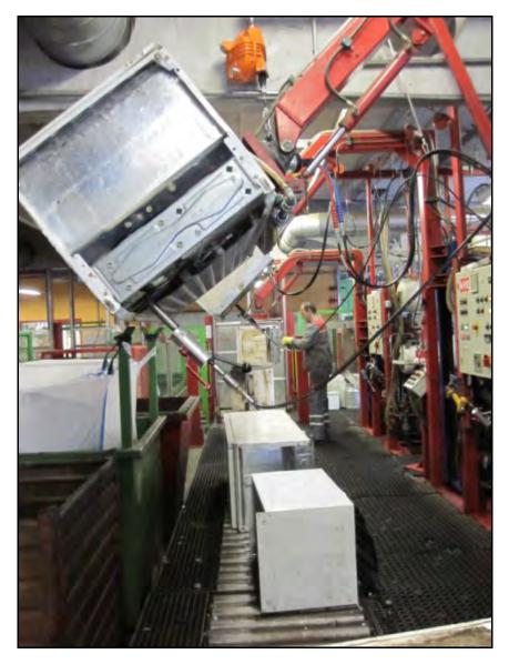
Picture 15 Step 1 of CFC recovery from refrigerators
