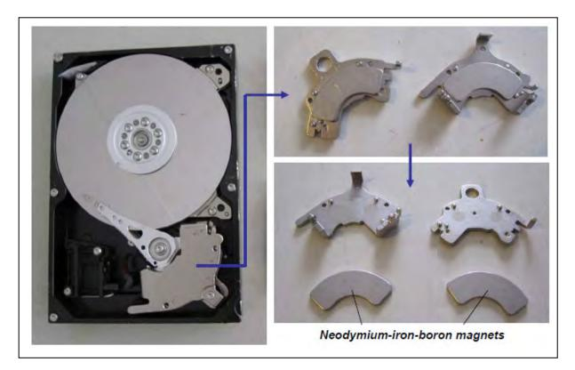
Picture 12 Neodymium-iron-boron magnets of hard drives
