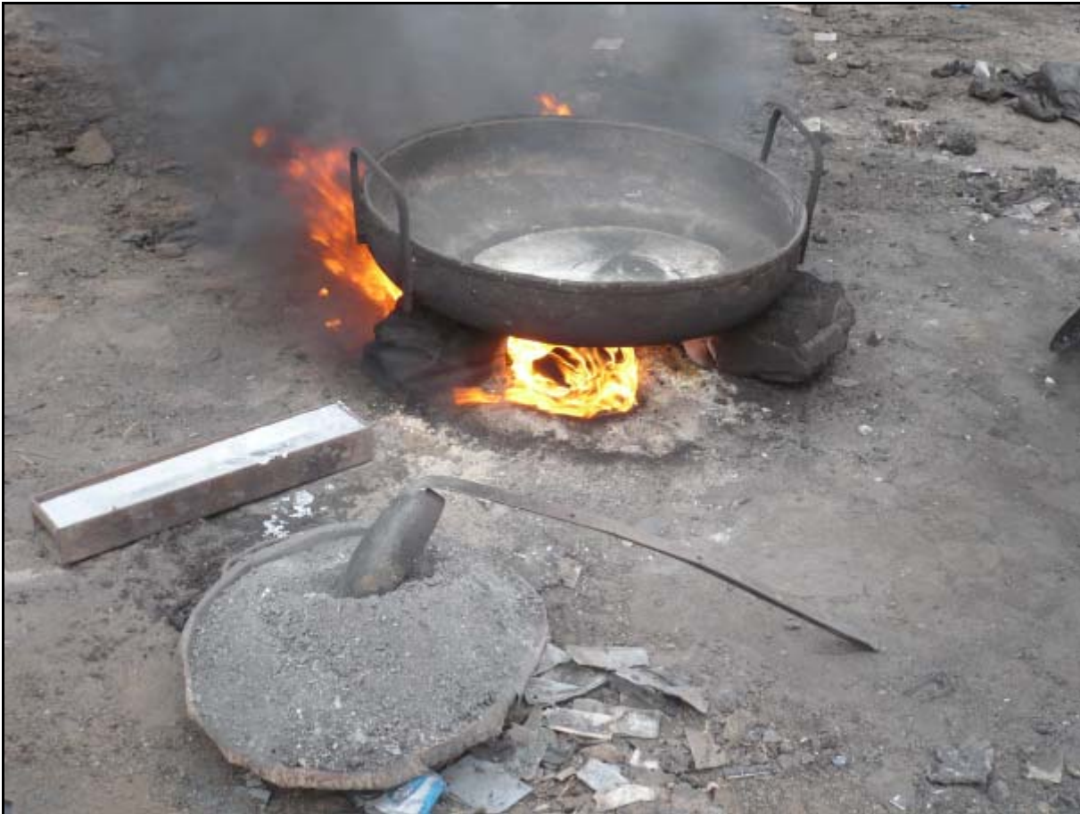
Photo 5 Recovery of lead at the Agbogbloshie Metal Scrap Yard, Accra (Source: Öko-Institut 2010)
