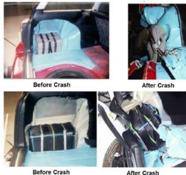
Figure 5 Potential impact of a crash on a component in the crumple zone of a vehicle.
