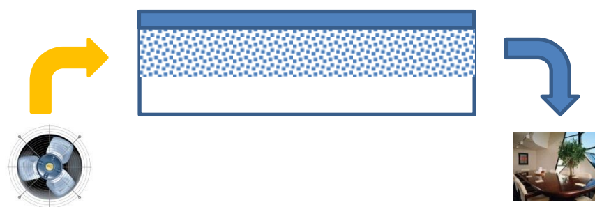
Figure 4 Principle of a single-stage direct evaporative cooler
