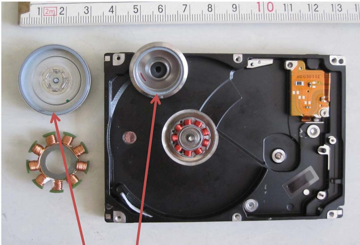
Ring magnets from spindle motors
