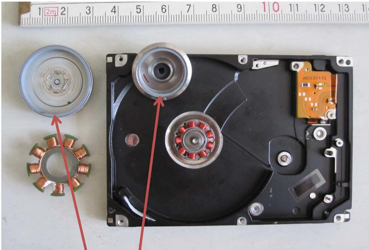
**Ring magnets from spindle motors**
