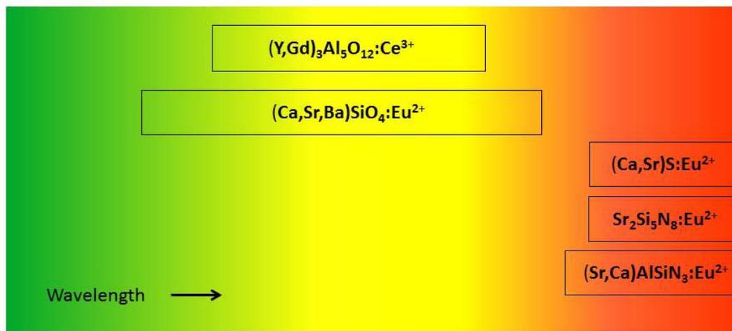
Normally 0.1 mg of the yellow luminescent substance is used for cold white LEDs. Table 27 shows the proportion of the individual elements in a yellow luminescent substance for the chemical compound  $(Y_{0.77}Gd_{0.2}Ce_{0.03})_3Al_5O_{12}$ .
