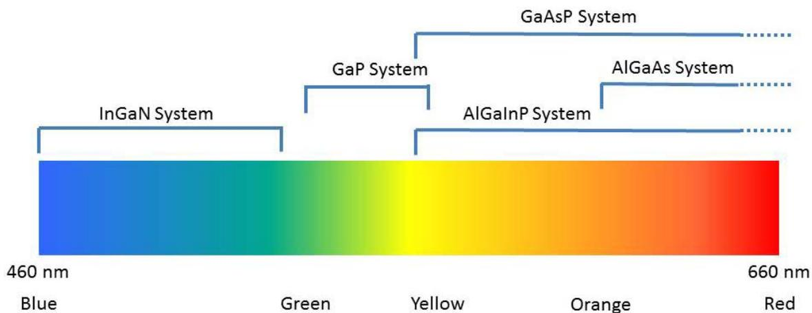
The larger the band gap, the shorter is the wavelength of the radiation emitted. However, radiant transitions only take place for specific values of some lattice parameters of the semiconductor used. These parameters are mainly produced by what are known as III-V
