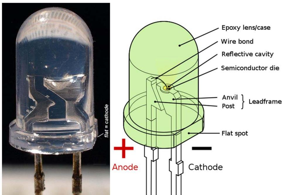
The semiconductor chip and luminescent material in an industrial LED are usually placed in a metal cup which bundles the light emitted in different directions and also serves to dissipate
