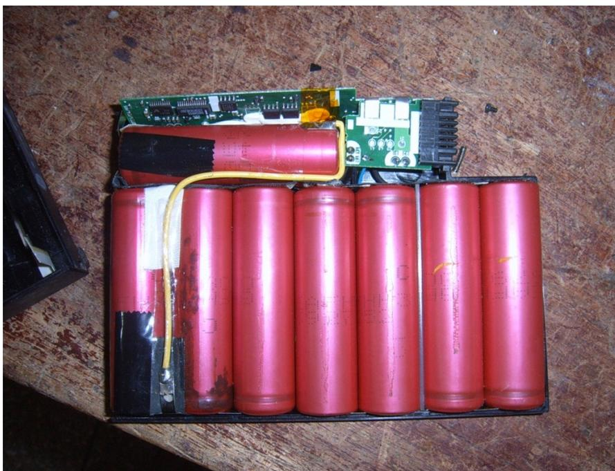
Other types of batteries such as e.g. NiMH are only of secondary importance in notebooks. The positive electrode in lithium-ion cells in notebooks consists of lithium cobalt oxide ( $\text{LiCoO}_2$ ) in most cases (Lauwigi et al. 2011). Although variations in the cobalt content can arise depending on the technology and design, Hagelüken & Buchert (2008) specify a mean
