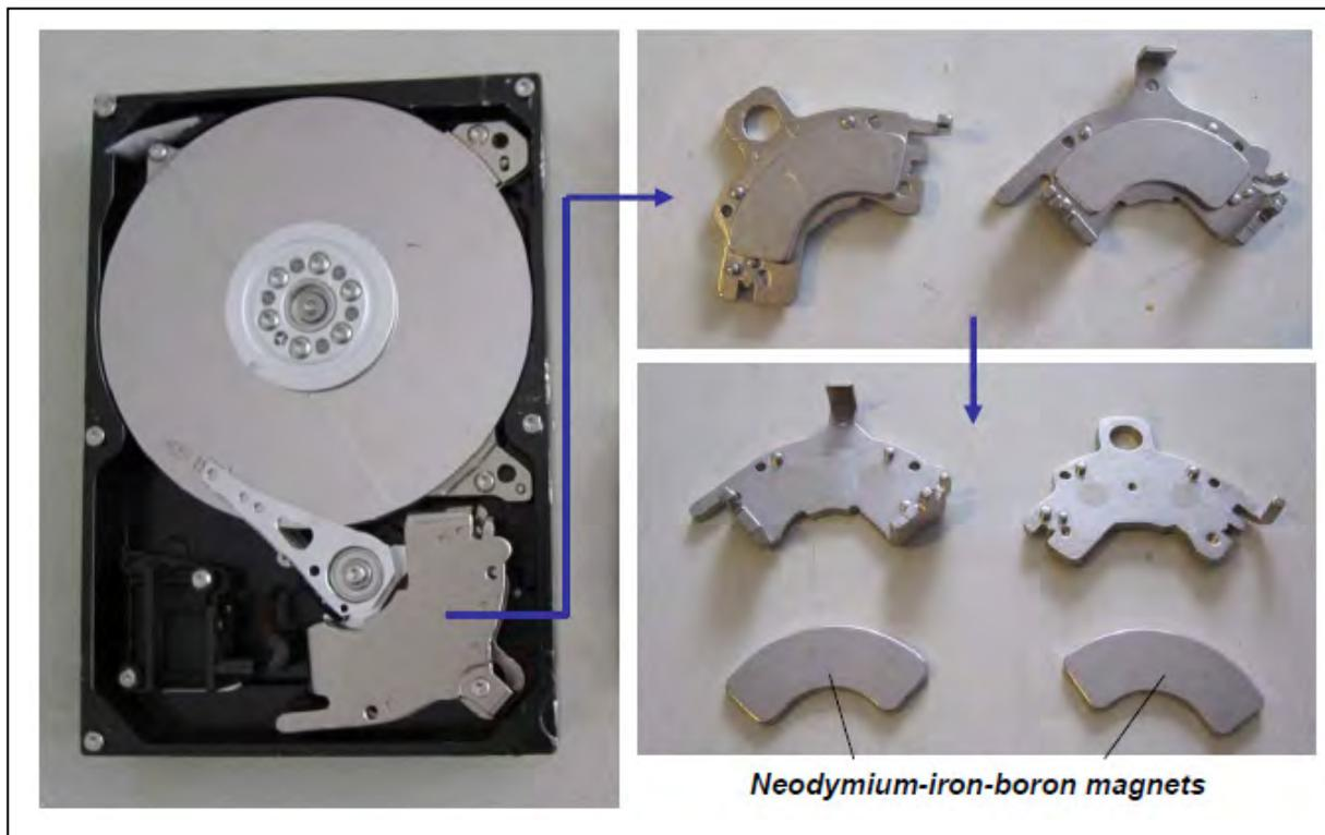
Picture 12 Neodymium-iron-boron magnets of hard drives
