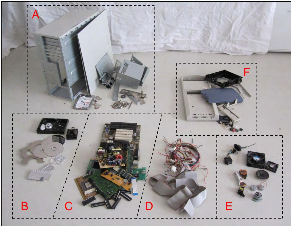
**A = Steel scrap      B = Aluminium scrap      C = High-grade precious metals fraction**
