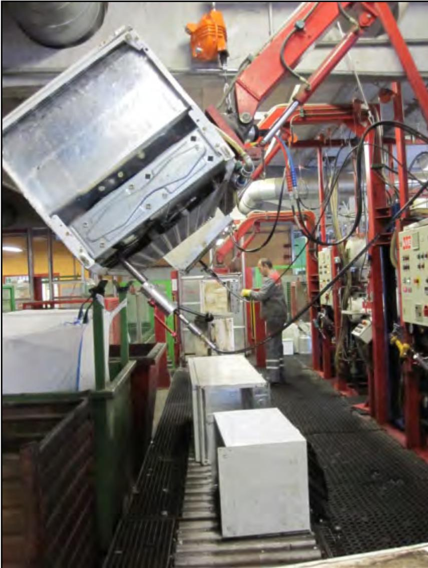
Picture 15 Step 1 of CFC recovery from refrigerators
