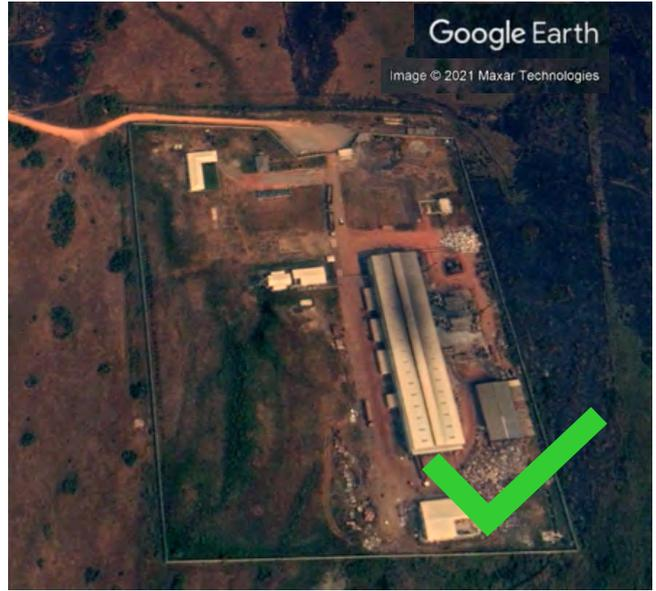
A ULAB recycling plant located in a designated industrial zone and well removed from residential areas. The surrounding land is not used for agriculture.
