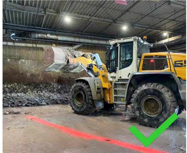
The sealed driver's cab in this vehicle engaged in charge preparation has a positive pressure HEPA filtered climate control system to minimise dust ingress. The charge preparation building is also under a negative pressure extraction ventilation system attached to a baghouse to prevent any dust emissions escaping from the building.
