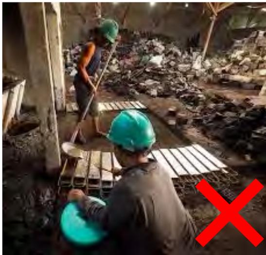
Molten lead is being cast manually to 25 kg ingots using a 3 kg ladle with a long handle. The lead is being poured close to the operator removing the dross rendering him directly in the line of fire should the molten lead spit or splash. In addition, the operators are not wearing appropriate PPE with insufficient footwear and eyes and skin exposed.
