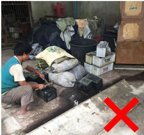
Batteries are drained manually at a collection point, and the electrolyte is drained to the public sewer. Acid and lead particles (dark colour) are severe environmental contaminants. Furthermore, the corrosive nature of the acid is a safety risk to the unprotected worker.
