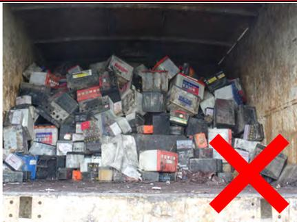
ULAB are packed into the back of a truck in any order. They are not upright or secured and could easily be damaged and leak during transit.
