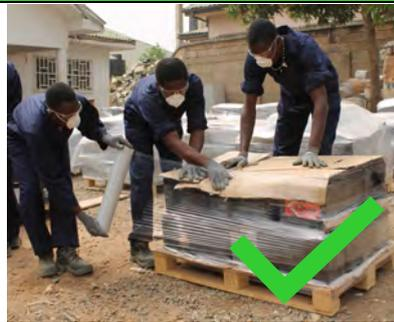
ULAB are sized and stacked upright on a solid pallet no more than 3 layers high. Thick cardboard is placed under and over each layer of ULAB, then strapped and shrink-wrapped.
