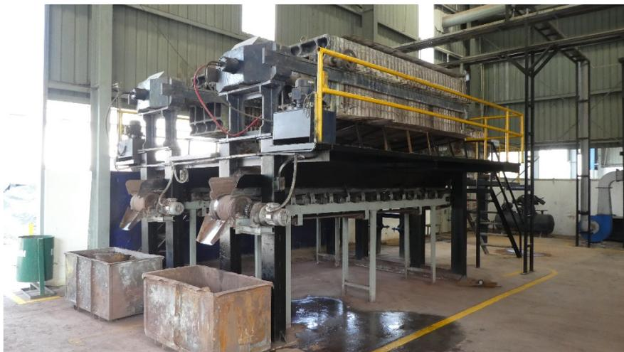
*Filter press removes suspended particulates from the electrolyte*
