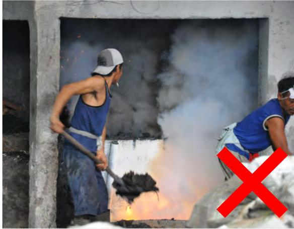
Operators using shovels for manual furnace charging. The operators are not wearing PPE. The operators are completely exposed to lead bearing dust, fume and any hot embers discharged from the furnace. The furnace extraction ventilation system fails to capture the dust and fume generated as the charge heats up.
