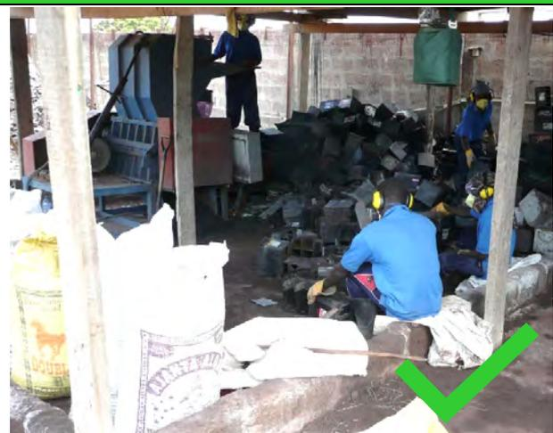
The plastic cases obtained from the battery saw breaking process are washed in an alkaline solution and water so that they are free of residual acid and battery paste before being fed into the case shedding machine to produce plastic chips that are sold to a plastics recycler.
