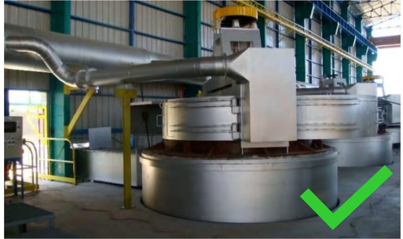
Integrated kettle refining complete with cover, extraction ventilation system connected to a baghouse, mixer, pump, inspection hatches for charging the kettle, sampling, reagent and alloy additions. This system also comes with automated de-drossing fitted internally. Dross is removed to a ventilated bin and all drosses are recycled internally. Operation of the kettle is from a remote workstation.
