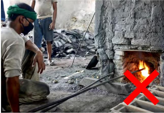
Hot fuming molten lead bullion is tapped from an unventilated port and poured into unventilated 25 kilo ingot moulds. Safety and occupational lead exposure risks will be high. Furthermore, operators are not equipped with effective PPE.
