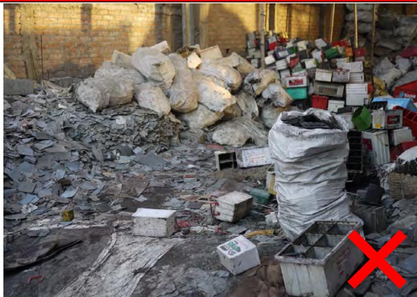
Pathways and emergency exits are blocked with debris and battery components, making any evacuation difficult and dangerous especially in the dark if the power fails.
