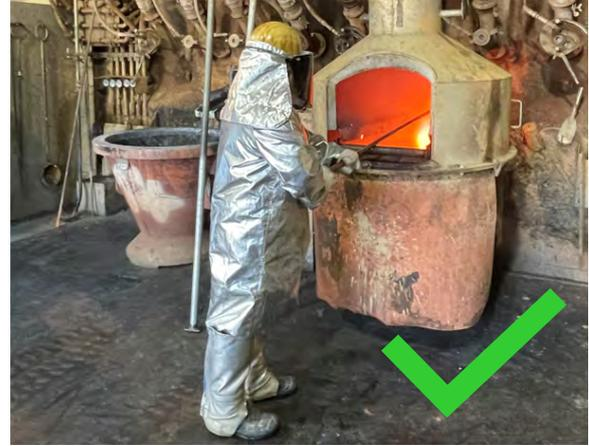
The operator is tapping the molten metal and slag into their respective pots with extraction ventilation hooding in place. The operator is wearing all the requisite PPE, including hard hat, face shield, respirator, overalls, and flame-resistant jacket and trousers.
