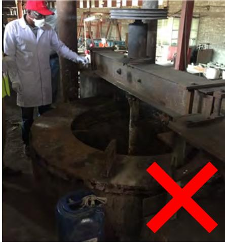
The refining kettle is set in the floor without a 1 metre skirt. This creates a hazard as the operator can fall into the molten lead bath. The kettle is not covered or attached to an extraction ventilation system.
