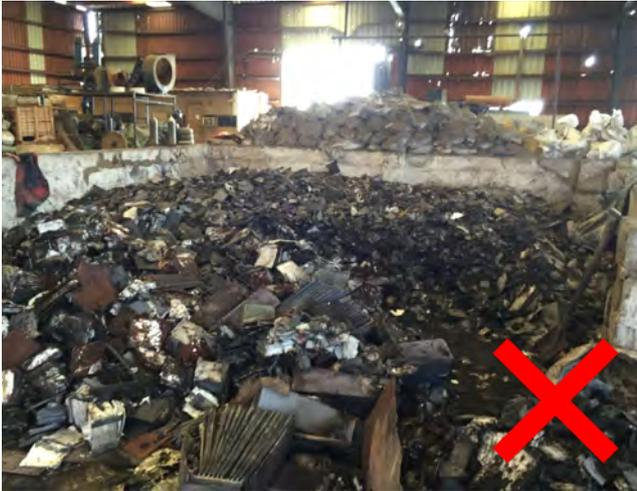
Charge material is stored in the facility, and not in a separated room or building. Fugitive emissions of lead dust are likely to contaminate the work environment. In addition, the building is open to the outside without any extraction ventilation or dust suppression.
