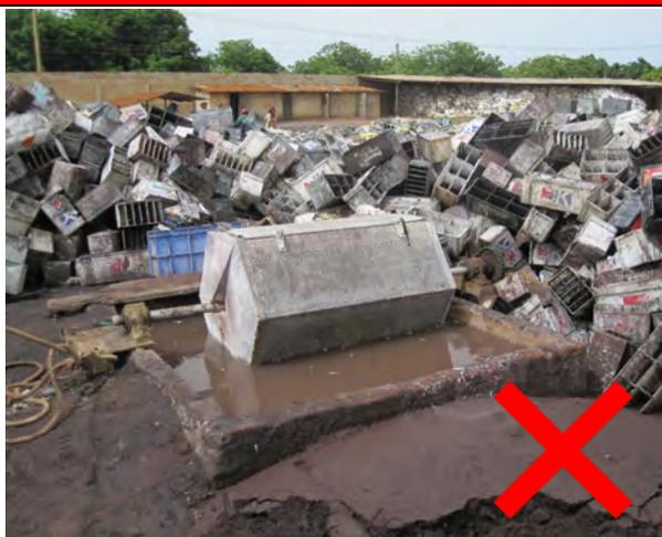
Plastic cases are washed in a rotating drum but the rinse water spills over and carries much of the lead and acid-containing residues to the surrounding area. Furthermore, the process is not sheltered from rainfall and is not situated on smooth and impermeable floor as required by A.2.5.
