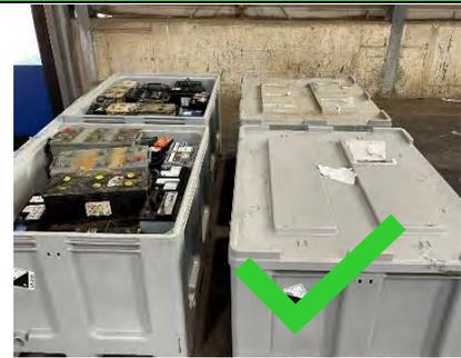
ULAB are placed upright in UN approved leakproof, fork truck friendly stackable plastic containers capable of holding 750 kg of ULAB. Containers come complete with a top cover.
