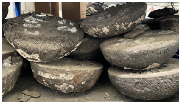
Figure 3-4: Alloy / matte as interim product of pyrometallurgical ULIB recycling
