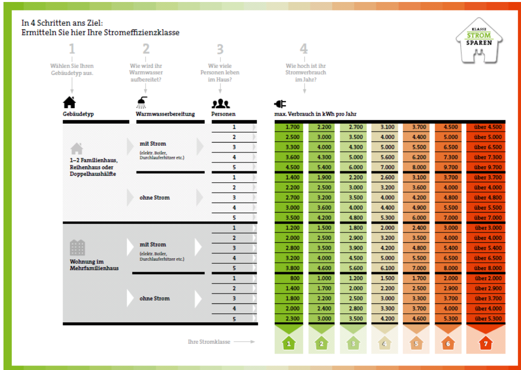
Figure 4: Self-analysis tool for households to determine power efficiency class. Source: Own illustration. Step 1: Type of house, Step 2: Hot water generation, Step 3: Number of persons in the household, Step 4: Power consumption in kWh/year.
