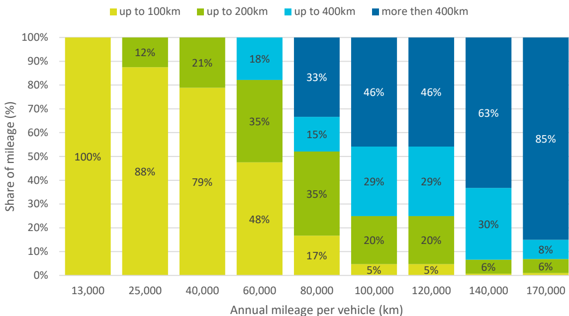
Figure 4-4: Weighting of the range classes within the annual mileage classes (maximum length of a single trip).
