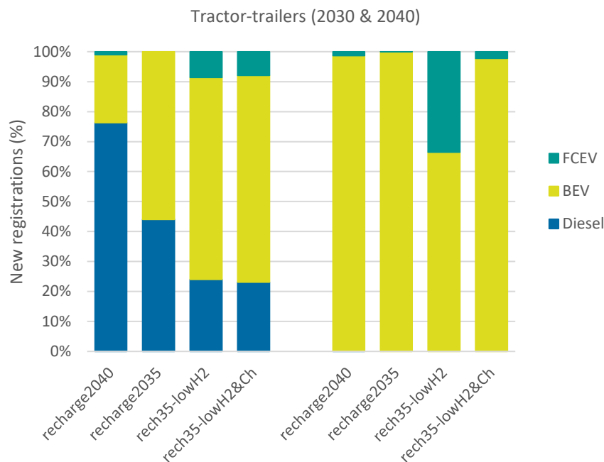
Figure 5-8: New registrations of tractor-trailers in 2030 and 2040 for the "BEV+FCEV" scenarios (variation of charging infrastructure availability as well as hydrogen and charging prices).
