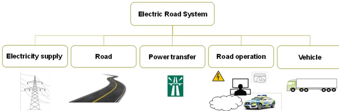
Figure 1: Overall system layout of ERS with five subsystems.
