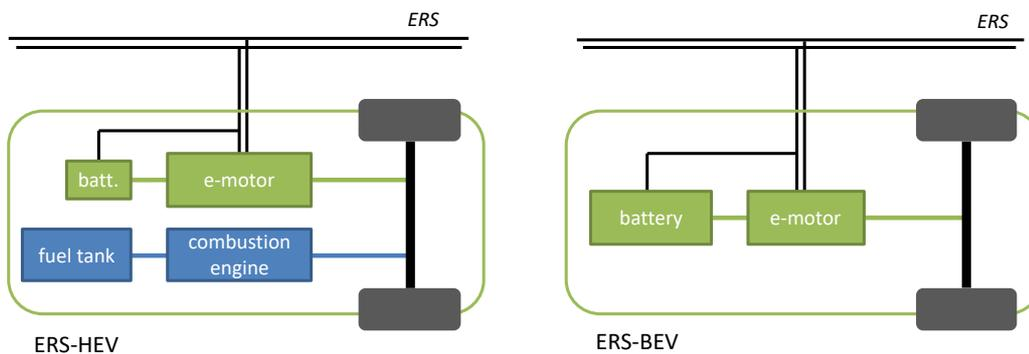
Figure 4: Schematic structure of the drive of an ERS-HEV and ERS-BEV.
