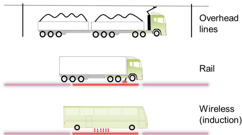
Figure 2: The three main concepts for road electrification and power transfer to moving vehicles.
