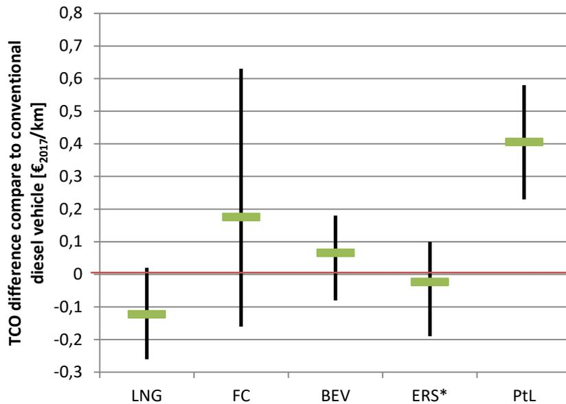
Figure 6: Differences in total cost of ownership (TCO) for different complementary drive systems and fuels compared to a fossil diesel vehicle 2020–2030 (\*ERS with overhead lines). PtL means Power-to-Liquids i.e. electrofuels. The green horizontal bars show averages and the black vertical bars shows intervals between different studies compiled by Plötz et al. [24].
