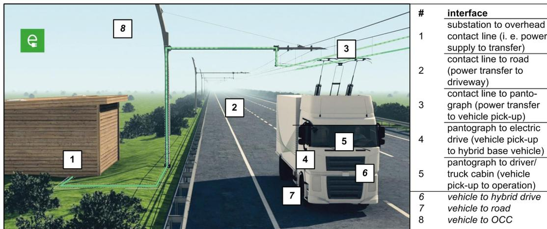
Figure 5: Technical overview using the example of overhead line ERS.
