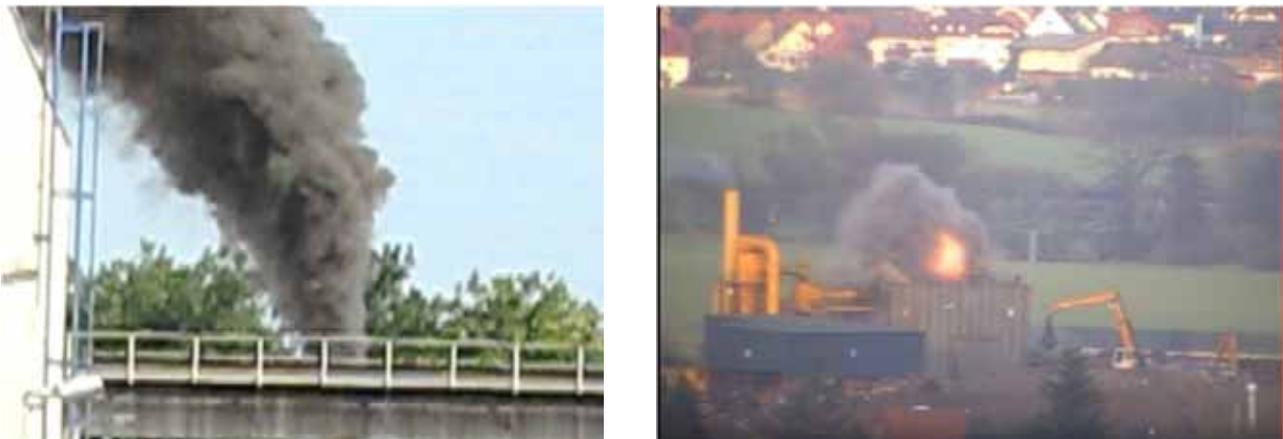
**Figure 10** Emission from a shredding plant during a deflagration (BREF WT, 2017)
