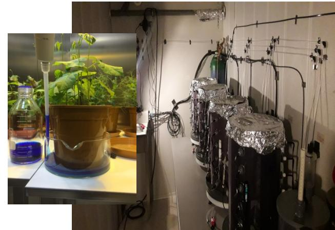
Different experimental arrangements for laboratory lysimeters
