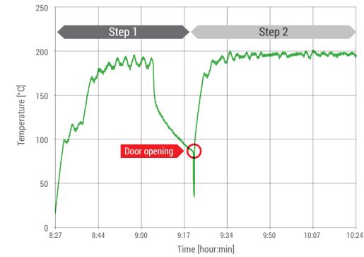
ANTICSS results of an oven model in ECO mode: energy consumption measurement (step 1) and temperature measurement (step 2)
