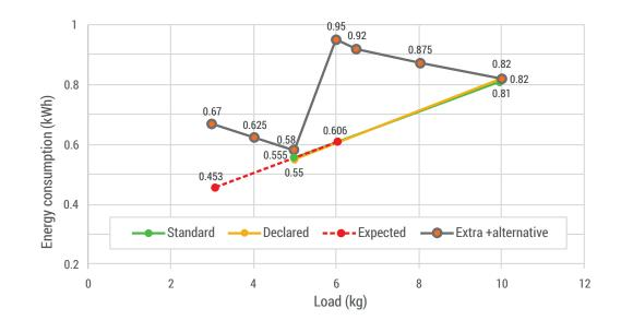
The increasing energy consumption at lower loads is remarkable as it could rather be expected that the energy consumption of the washing machine would rise with increasing wash load or getting lower with smaller loads (note: a linear dependency of the washing machine's energy consumption to the load is an approximation introduced by the ANTICSS project for sake of simplicity although it is well known that the usual relation is not linear).
