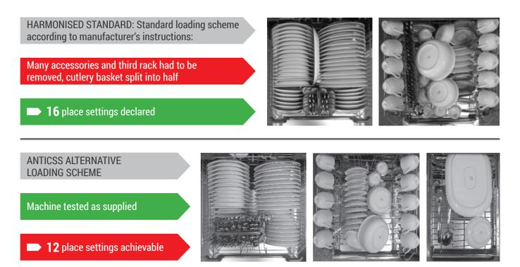
ANTICSS testing of a dishwasher model: harmonised standard and modified loading scheme
