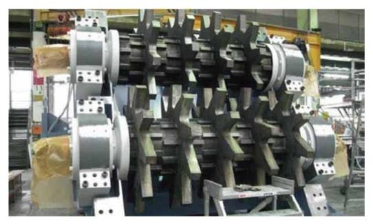
Figure 8 Example of a pre-shredder; Source: BREF WT 2017
