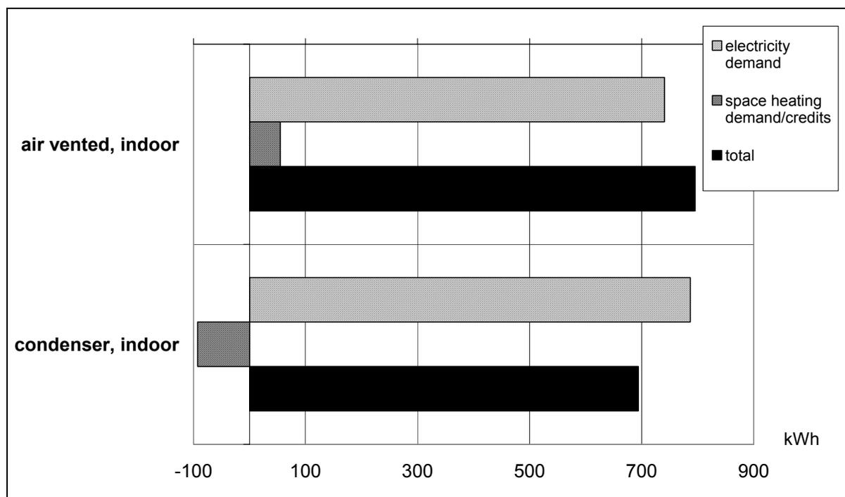
Fig. 8.1 structure of the CED of indoor drier use under real life conditions (example: *Germany indoor base case*)
