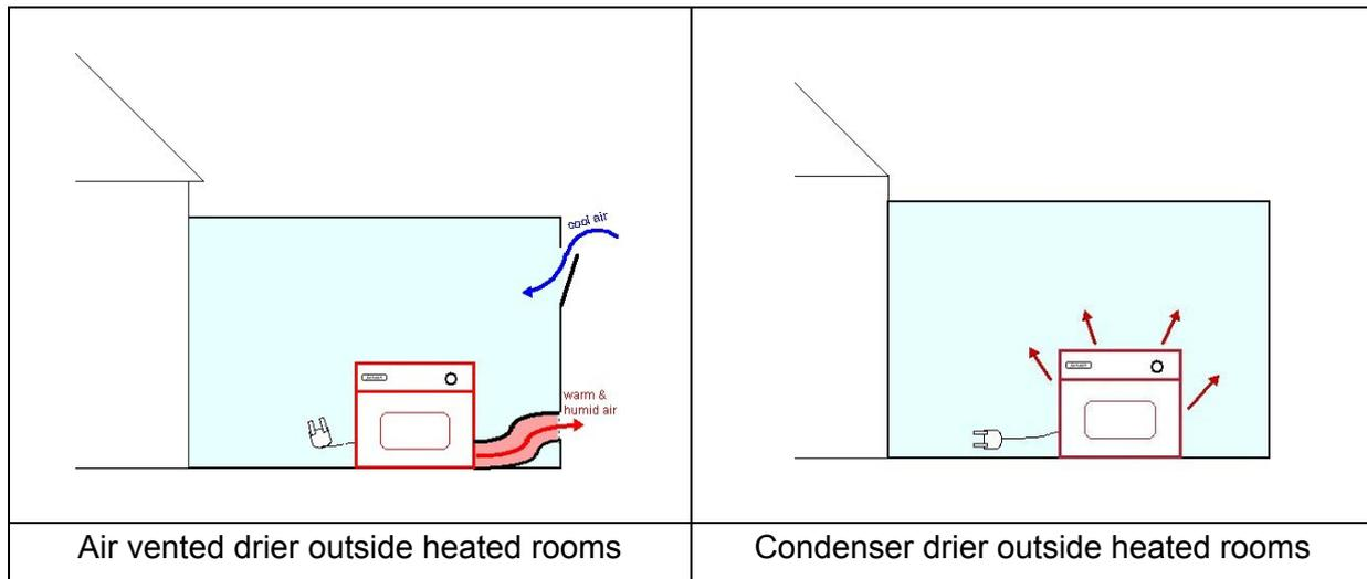
Fig. 3.3 to 3.4: drier use outside heated rooms
