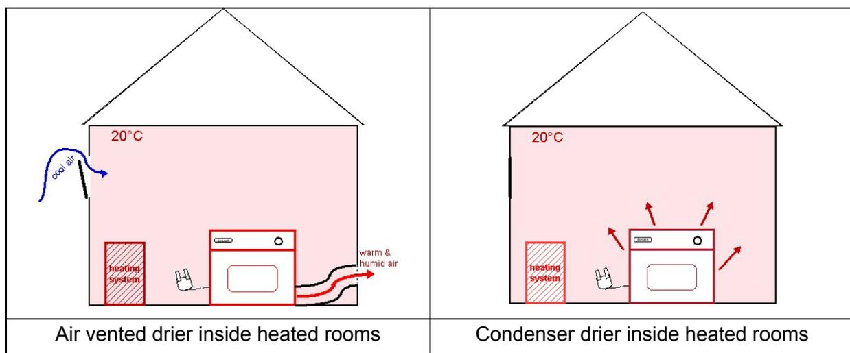
Fig. 3.1 to 3.2: drier use insite heated rooms
