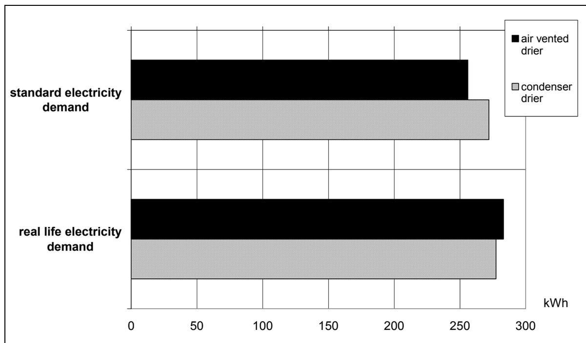
Fig. 8.3 standard and real life electricity demand of air vented and condenser driers (Germany outdoor)
